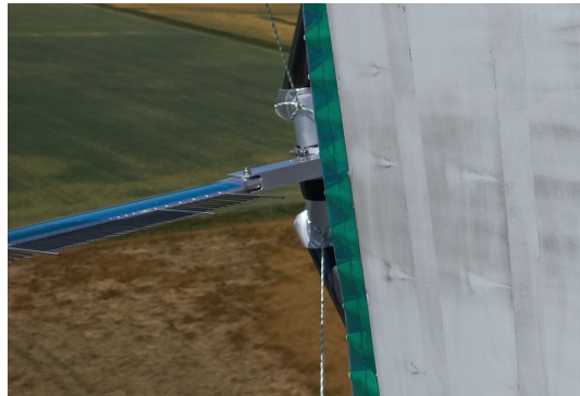
(c) Close-up view of serrations covered with a tape to avoid spanwise velocity deficit variations.
