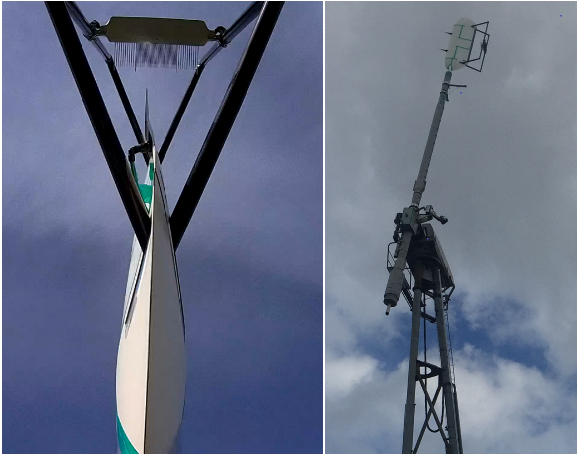
Figure 2. Left: The wake rake attached to the 2 m span blade section with carbon fiber circular tubes fastened inside the blade section to the aluminum frame. Right: The blade section on the 10 m long rotating boom during the RTR tests.
