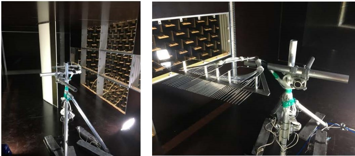
Figure 1. Photos of the set-up of the test wake rake in the Poul la Cour wind tunnel at DTU. The wake rake was installed behind a blade section with a span of 2 m, a 1 m chord and with a morphing trailing edge flap.
