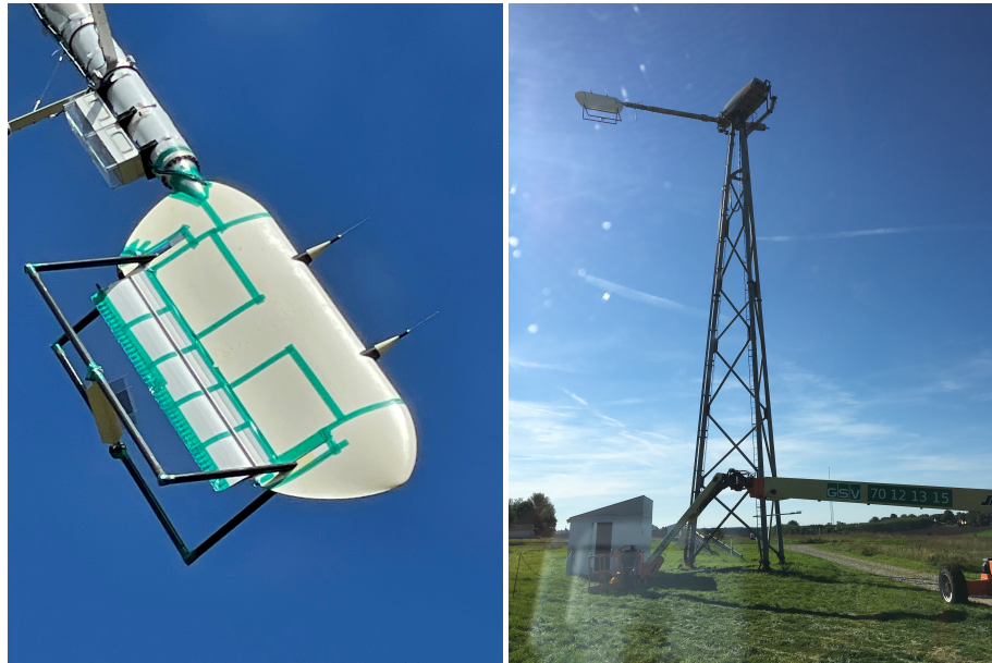
Figure 3. Left: The wake rake attached to the 2 m span blade section with carbon fiber circular tubes fastened inside the blade section to the aluminum frame. Right: The blade section on the 9m long rotating boom during the RTR tests.
