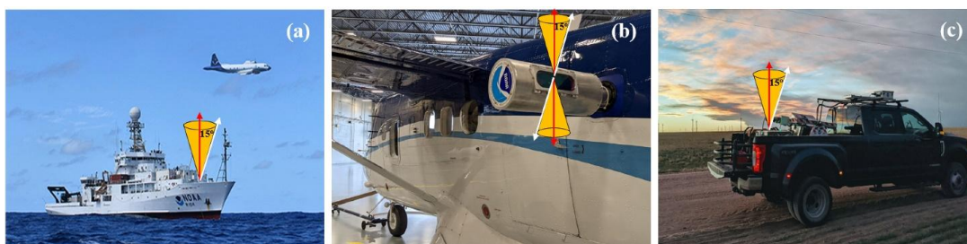
147 148 Figure 1. NOAA/CSL Mobile Doppler Lidar Systems: (a) Ship-based; (b) Aircraft-based; (c) Truck-based.
