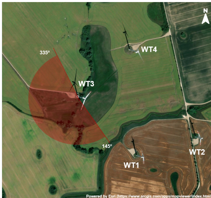
Figure 2. Layout of the test site showing turbine positions. The digital shadow is evaluated on WT3. The red sector indicates the wind direction range during the measurement period, covering both simple and complex inflow conditions.
