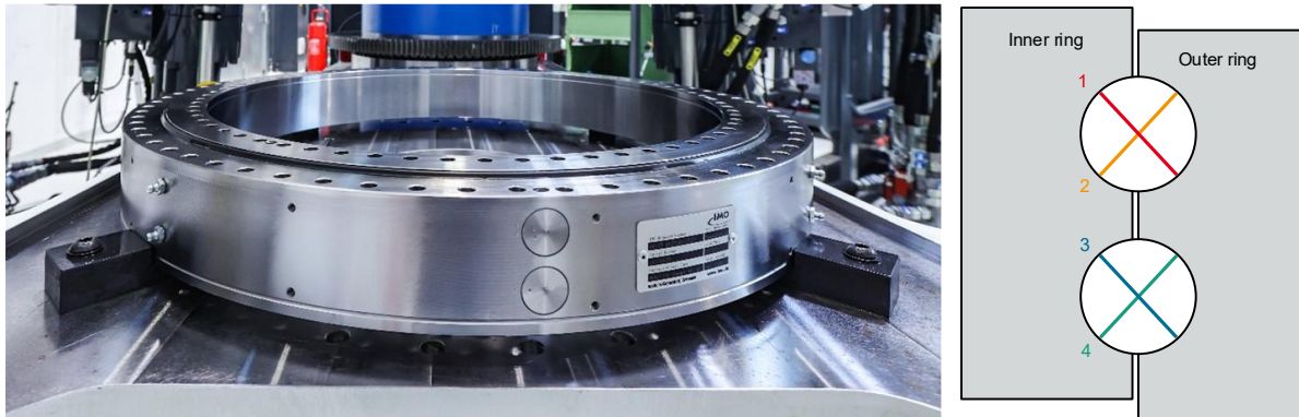
Figure 1: Double-row four-point contact ball bearing (left) (© Fraunhofer IWES/Ulrich Perrey) and load carrying diagonals (right).
