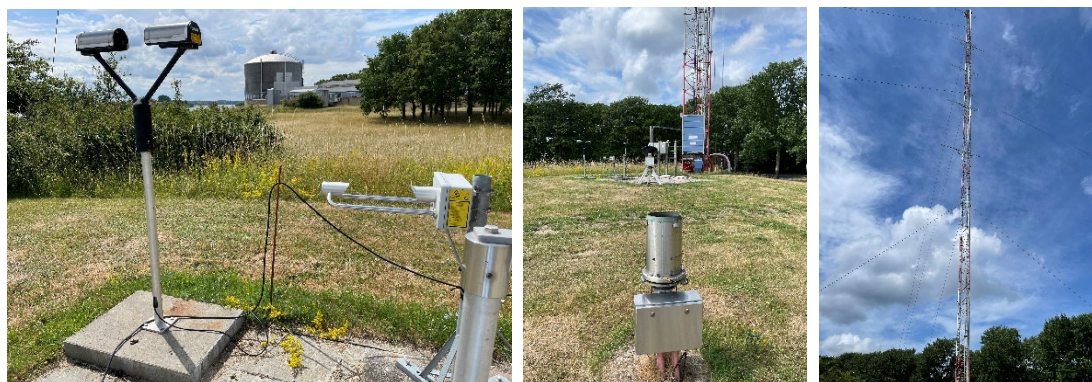
Figure 2. Photos from left Parsivel 2 and Thies, rain gauge, and meteorological mast at Risø site.
