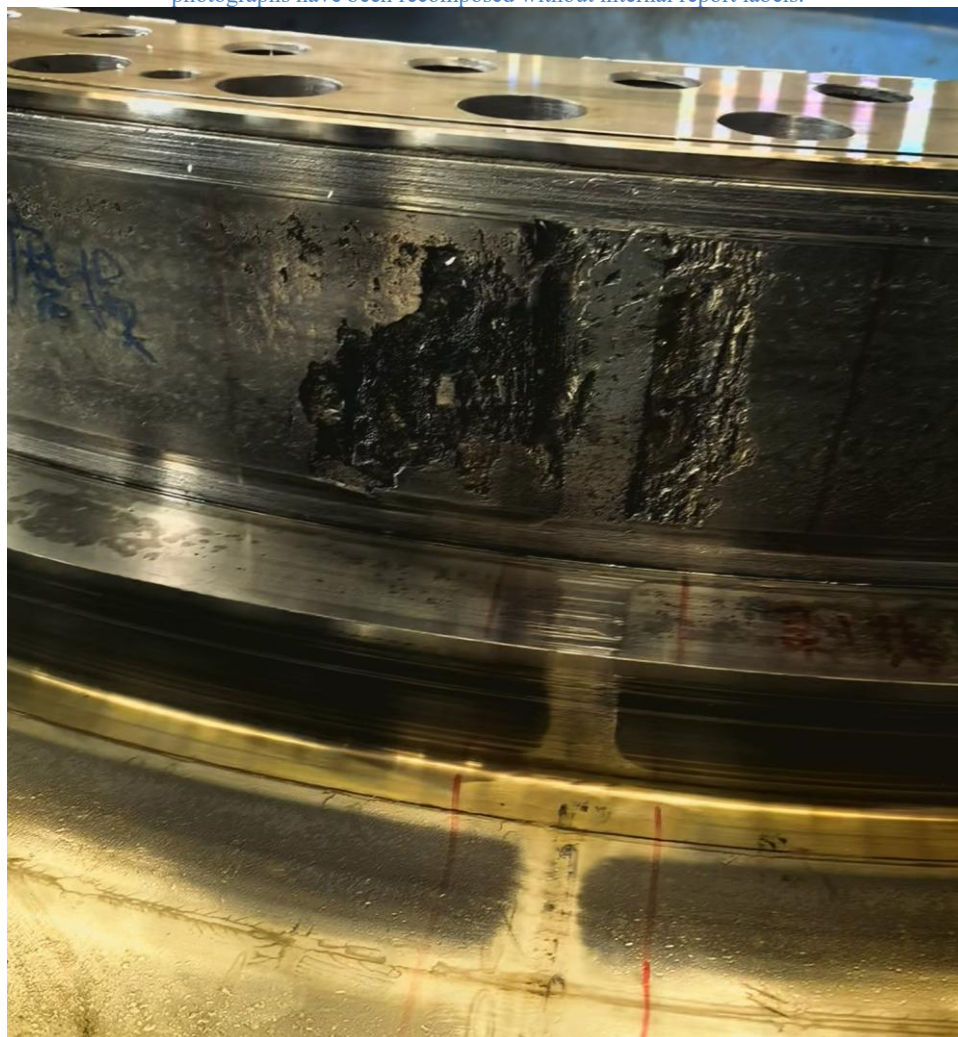
Figure 3: Field photograph comparing severe radial outer-raceway spalling with comparatively intact adjacent raceway regions. The image has been re-encoded without report overlays.
