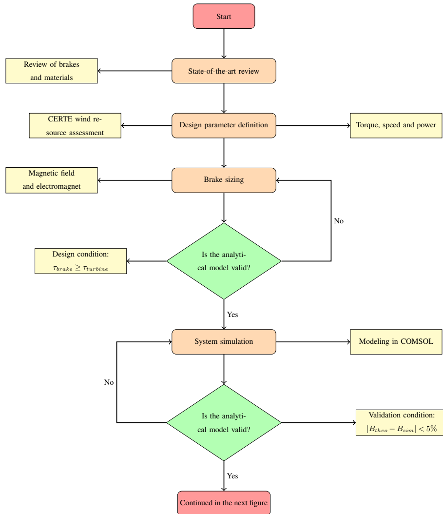
Figure 1. Methodology (Part 1): theoretical analysis and numerical validation. Source: own elaboration.
