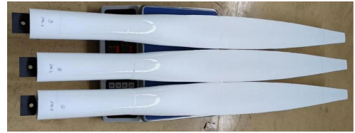
Figure 6. Model blade design and manufacture: (a) aerodynamic geometry design; (b) sizing and calibration of the carbon-fibre spar within the local airfoil envelope, retaining a clearance margin at each section; (c) manufacture of the carbon-fibre spar; (d) machining of eight PMI52 foam segments with internal openings and assembly onto the spar; and (e) application of a heat-shrink covering to complete the blade surface. Red outlines and shaded rectangles in (b) denote the airfoil boundaries and spar cross-sections, respectively.
