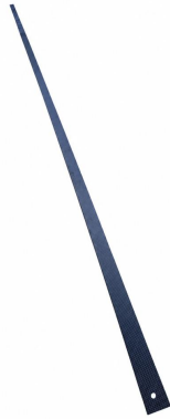
Figure 6. Model blade design and manufacture: (a) aerodynamic geometry design; (b) sizing and calibration of the carbon-fibre spar within the local airfoil envelope, retaining a clearance margin at each section; (c) manufacture of the carbon-fibre spar; (d) machining of eight PMI52 foam segments with internal openings and assembly onto the spar; and (e) application of a heat-shrink covering to complete the blade surface. Red outlines and shaded rectangles in (b) denote the airfoil boundaries and spar cross-sections, respectively.
