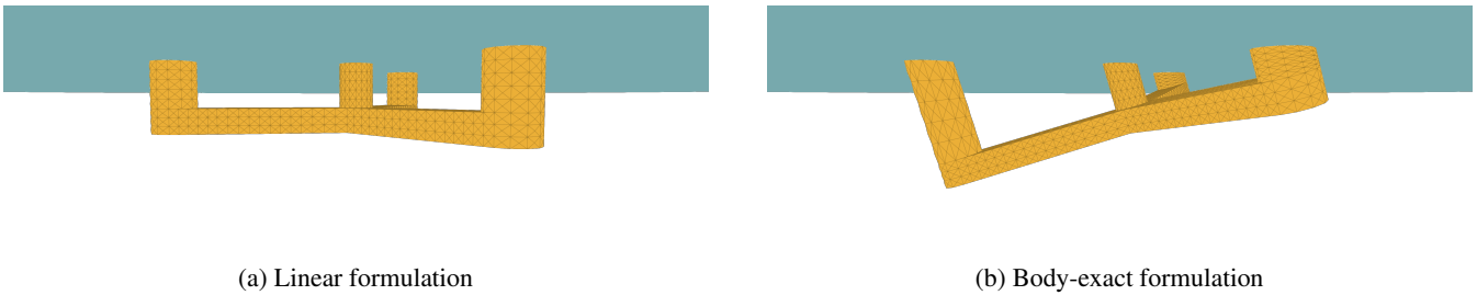
Figure 1. UMaine VoltturnUS-S geometry for the linear and body-exact formulations at a pitch motion of \theta_0 = 6^\circ .
