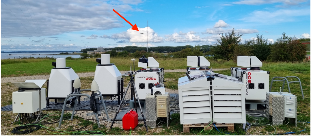
Figure 5. Photo of the pre-campaign lidar tests at Risø test station. A telescopic sight is fitted to the system in the center to help align the scan head with the met-mast and drone. The drone is flying and is visible in the center of the image at the red arrow.
