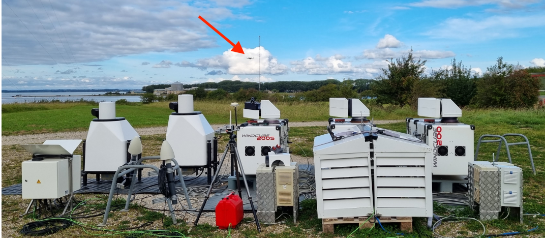
Figure 5. Photo of the pre-campaign lidar tests at Risø test station. A telescopic sight is fitted to the system in the center to help align the scan head with the met-mast and drone. The drone is flying and is visible in the center of the image at the red arrow.
