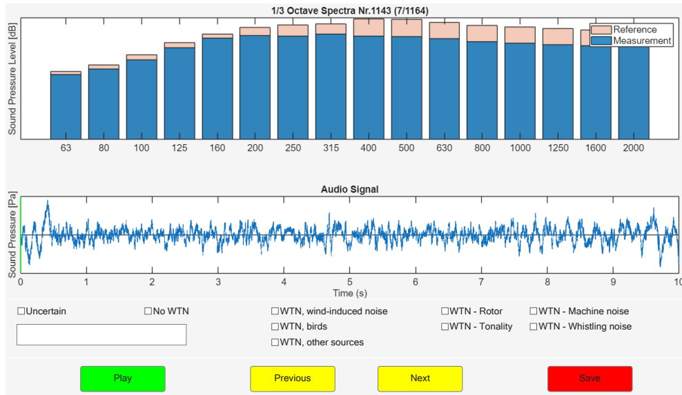
Figure A1. Graphical user interface (GUI) of the listening test used for the evaluation of wind turbine sounds. The GUI displays the time course of the audio signal and the corresponding sound spectrum, together with a reference spectrum characterising WTN.
