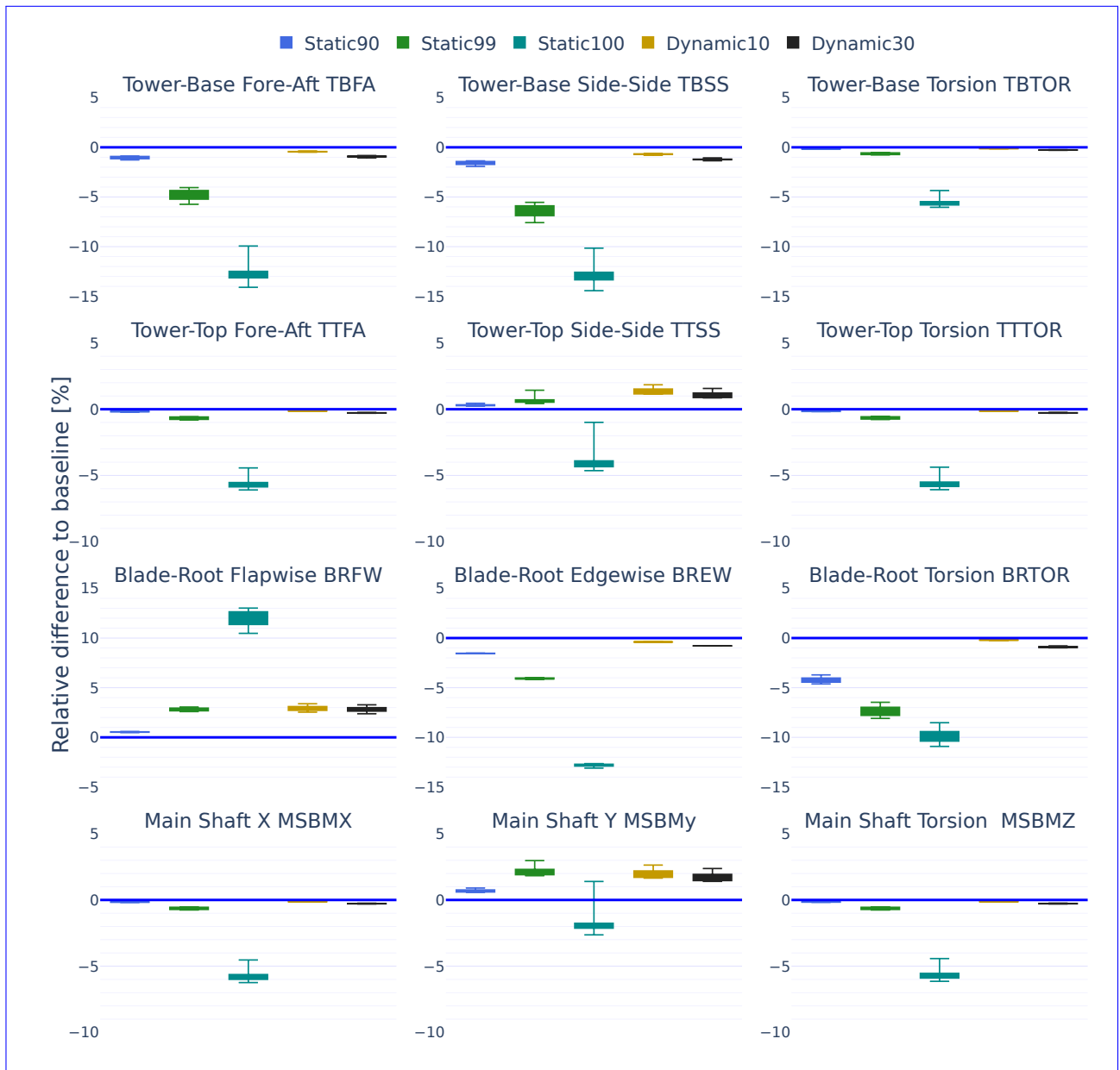
Figure 11. Relative differences in cumulative fatigue damage with respect to the baseline case for the full evaluation period. Each subplot corresponds to one load channel, and box plots summarize the distribution across turbines for the evaluated strategies. The box spans the 25th to 75th percentiles, and the whiskers denote the minimum and maximum values.
