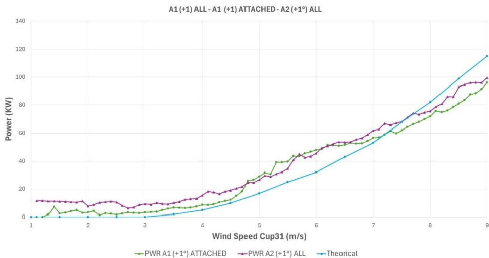
Figure 13 - A1(pitch +1°) & A2(pitch +1°) power curve filtering according to the Attached / Detached criteria
