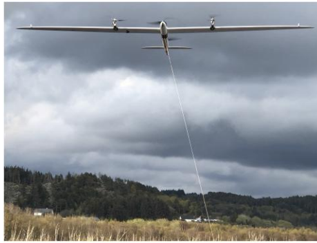
Figure 1. Aerial component of Kitemill's KM1 system.
