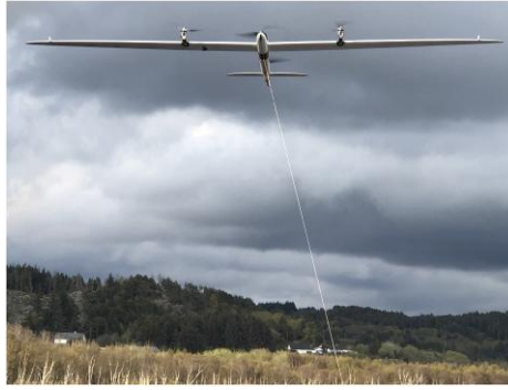
Figure 1. Aerial component of Kitemill's KM1 system.
