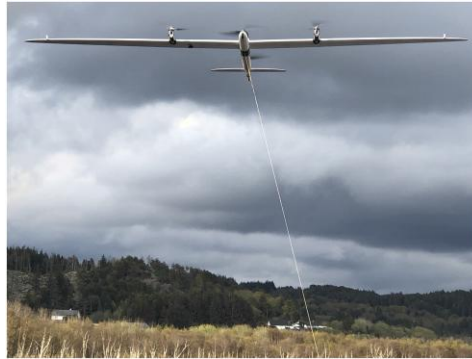
Figure 1. Aerial component of Kitemill's KM1 system.
