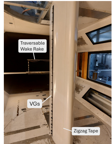
(b) Airfoil model in the test section
