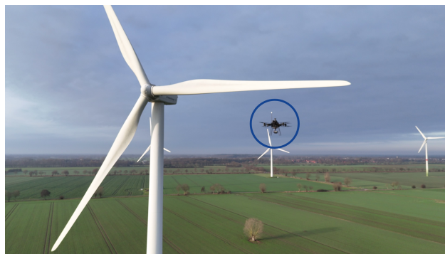
Figure 5. UAV in flight during an in-field measurement on an operational wind turbine. The UAV is highlighted by a blue circle and positioned at the pressure side of the rotating rotor, illustrating the measurement geometry and stand-off configuration used during the experiments.
