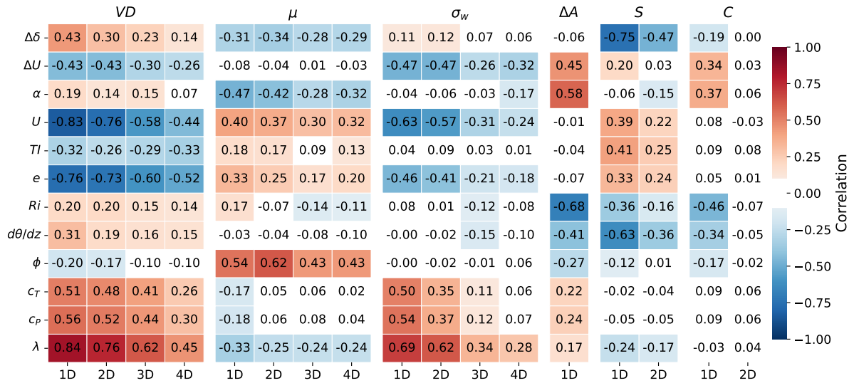
Figure 8. Heatmap showing correlations of wake characteristics (columns) against meteorological and turbine variables (rows) for down-stream distances 1-4 D , correlations for \Delta A solely at 1 D , and S and C at 1-2 D .
