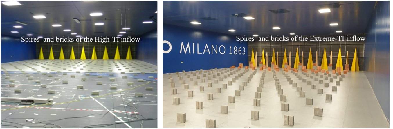
Figure 2. Spires and bricks used to simulate the High-TI boundary layer (a). Spires and bricks used to simulate the Extreme-TI boundary layer (b).
