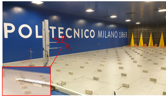
Figure 5. Traversing system equipped with two CTA probes, each one measuring the three components of the velocity vector \mathbf{u} along the longitudinal ( u_x ), lateral ( u_y ), and vertical ( u_z ) directions.
